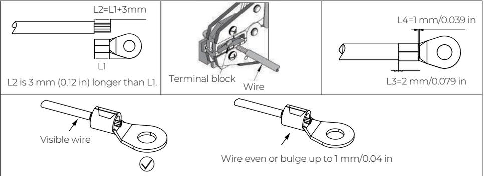
**Step 3:** Fix the OT terminal with M5 screw at the position shown in the figure below.
