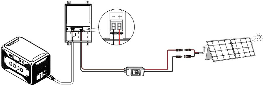
Step 1: Make sure the PV switch is in the "OFF" position.
