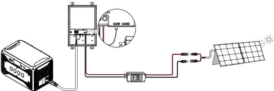
**Note:** When using BLUETTI battery packs, make sure the Ethernet cable is securely connected to the CAN communication port.
